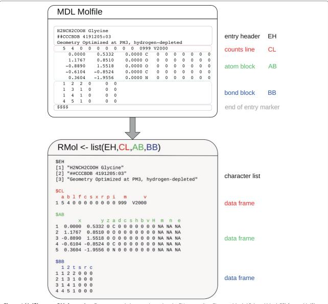
Figure 1 Molfile <—> RMol mapping. Four structural elements (entry header EH, counts line CL, atom block AB, bond block BB) from a Molfile are transformed to list elements of an RMol object. Column labels of the RMol data frames CL, AB, BB are named according to the CT (Chemical Table) file specifications [23].
